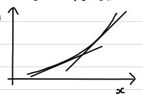
Concave upwards: curve lies above its tangent at all points in the interval
