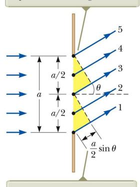
The path difference between rays 1 and 3, rays 2 and 4, or rays 3 and 5 is  $(a/2) \sin \theta$ .
