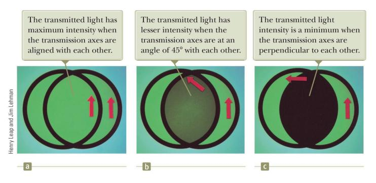
On the left, the transmission axes are aligned and maximum intensity occurs. In the middle, the axes are at 45° to each other and less intensity occurs.
