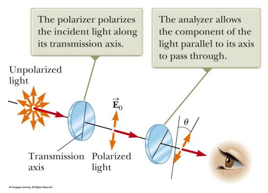
The most common technique for polarizing light.
