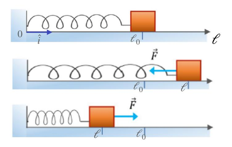
We consider an object of mass m on a frictionless horizontal surface attached to the end of a spring whose rest length is  $\ell_0$ . When the block is displaced from its equilibrium position, the spring exerts a restoring force  $\overrightarrow{F} = F(\ell)\hat{i}$ .
