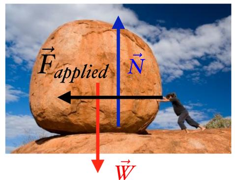
*Ist step*: make a diagram with all the forces acting on the boulder
